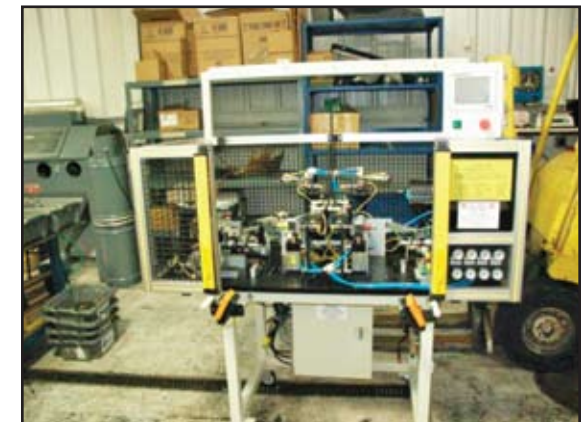
Production Recliner Function Computer Controlled Cycle Test Machine
