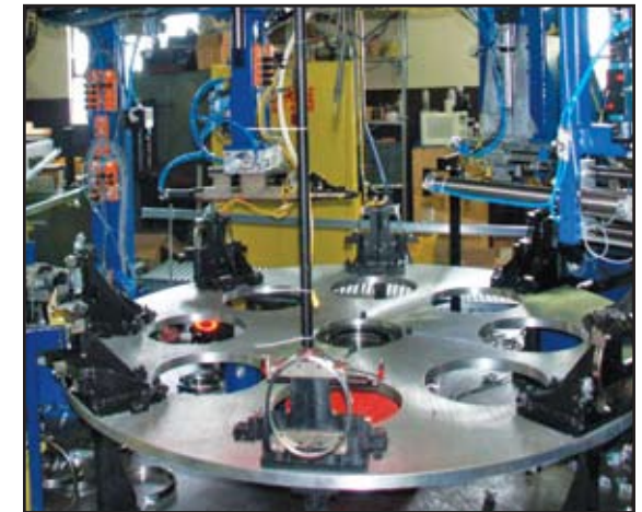
8 Stations Dial Assemble Machine with Vision Inspection Cameras
